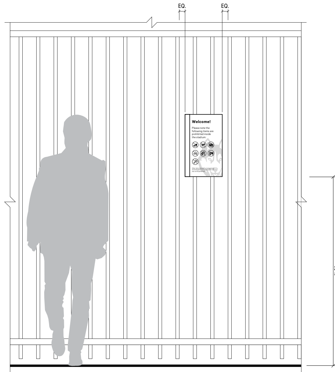
1 Installation Elevation - Sign Type Q2 3/4" = 1'-0"
